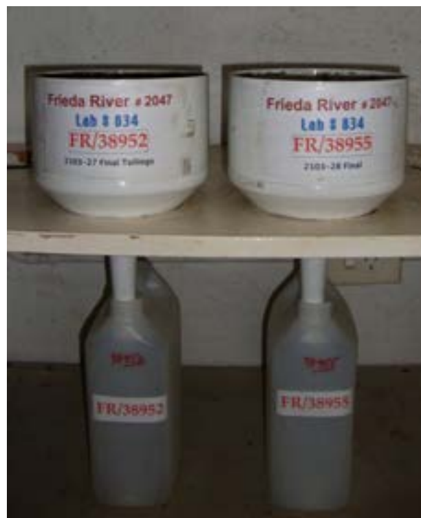
FIGURE 6: Side view of column leach tests involving tailings
