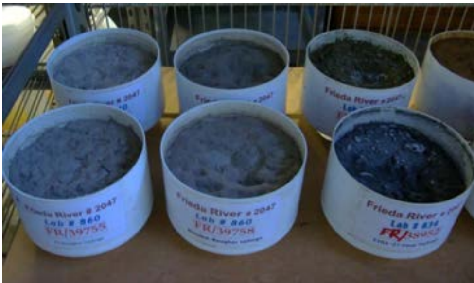
FIGURE 7: Top view of column leach tests involving tailings
