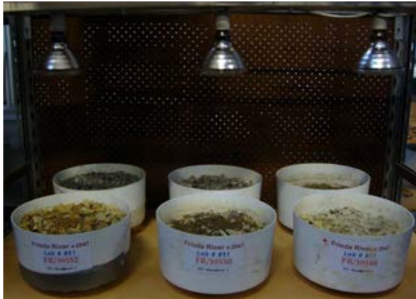
FIGURE 5: Larger column leach tests involving HIT waste rock samples
