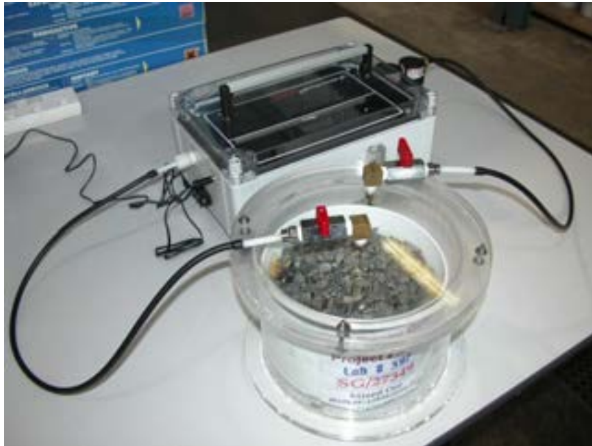
FIGURE 8: Sulfide oxidation chamber (SOC) used to measure intrinsic oxidation rate
